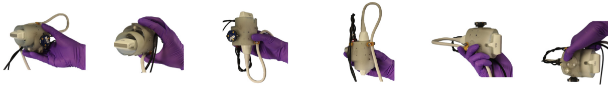
Fig. 3. Measurements were taken in six different orientations to compensate for the weight of the ultrasound probe.
