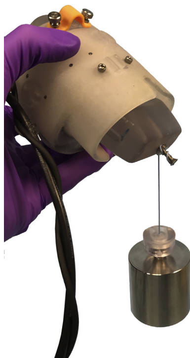
Fig. 6. A weight was suspended from the ultrasound mock probe tip after gravity compensation was performed. Measurements were taken in ten arbitrary orientations.
